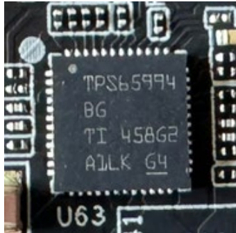
Optical image showing the Controller Texas Instruments Semiconductor Part Number TPS65994
