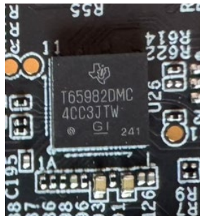
Snapshot of Texas Instruments TPS65982 A chip inside the CalDigit TS5
